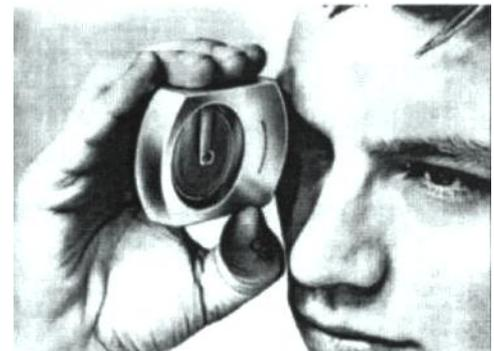
7. Aim with your left eye at the object to be measured (like the top of a tree)
